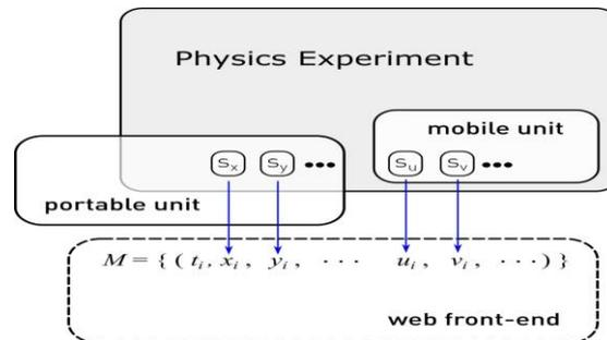
Figure 1: A conceptual diagram showing the main components of the system. It comprises a mobile unit that includes several sensors ( $s_u; s_v; \dots$ ) controlled by an Arduino board and a portable unit with a Raspberry Pi that communicates with the Arduino and establishes a Wi-Fi network. It can also host additional sensors ( $s_x; s_y; \dots$ ). The measurements of all the sensors can be transferred into the users' devices as series of vectors
