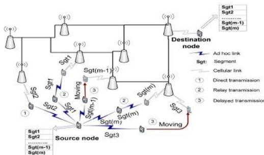
Fig. 2: Data transmission in the DTR protocol.
