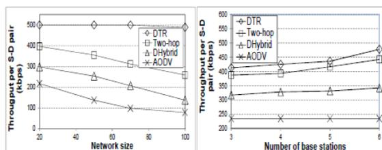
Fig. 6: Throughput vs. network size (simulation). Fig. 7: Throughput vs. number of BSes.
