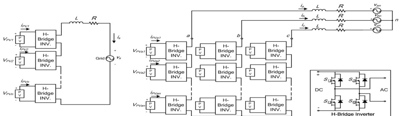
Fig. 2. Topology of the modular cascaded H-bridge multilevel inverter for grid-connected PV systems.
