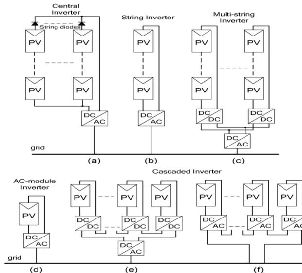
Each phase consists of  $n$  H-bridge converters connected in series, and the dc link of each H-bridge can be fed by a PV panel or a short string of PV panels. The cascaded multilevel inverter is connected to the grid through  $L$  filters, which are used to reduce the switching harmonics in the current.
