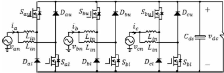
Circuit diagram of the proposed three-phase ac–dc dual boost rectifier.
