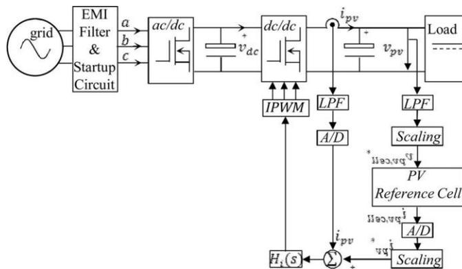
FIG Control strategy block diagram for the three-phase dc-dc converter.
