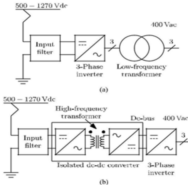
Figure. 1. Schematic of an APU. (a) Conventional APU. (b) Proposed APU.
