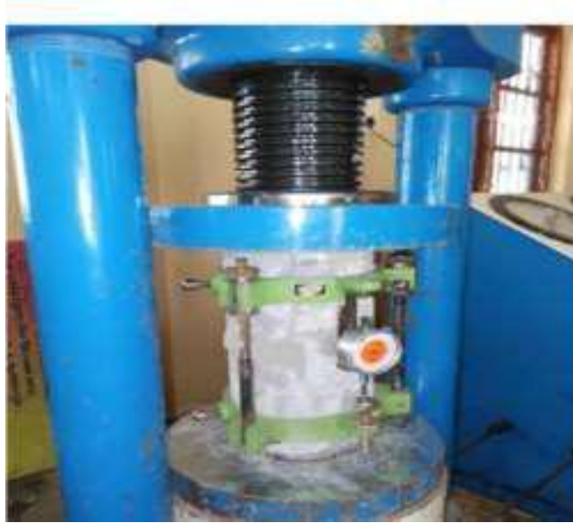
Fig2: Cylinder Specimen Placed in CTM Strain dial gauge
